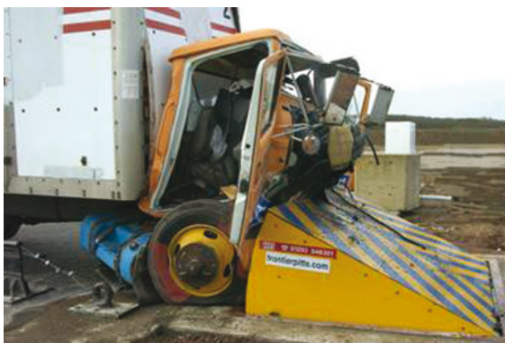
First Terra Blocker impact test in 2004. K12 L3 test with a 6800kg American truck travelling at 80kph (50mph). Fully functional after impact.
