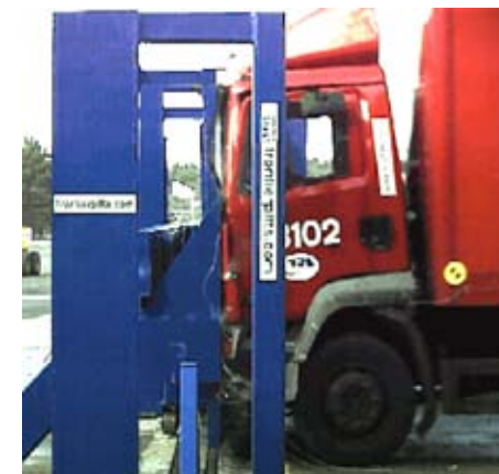
PAS 68 Terra Gate impact test in the half open position
