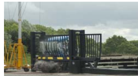
Terra Beam design in based on the PAS 68 Terra Sliding Cantilevered Gate
